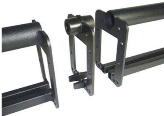
Moulded in Acetyl the Sixtrack Spigot Plate has been designed to aid track installation and alignment. The Spigot Plate simply fits between each track joint locating the top and bottom rails ensuring they are perfectly aligned to provide a smooth running track system.
